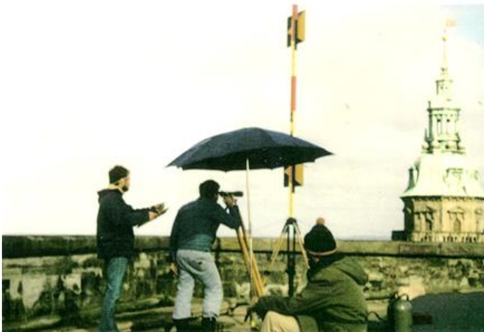
Figure 11: Trigonometric water crossing over Öresund between Kronborg and Pålsjö klint in 1981, using Wild N3, a joint project between KMS and LM.
