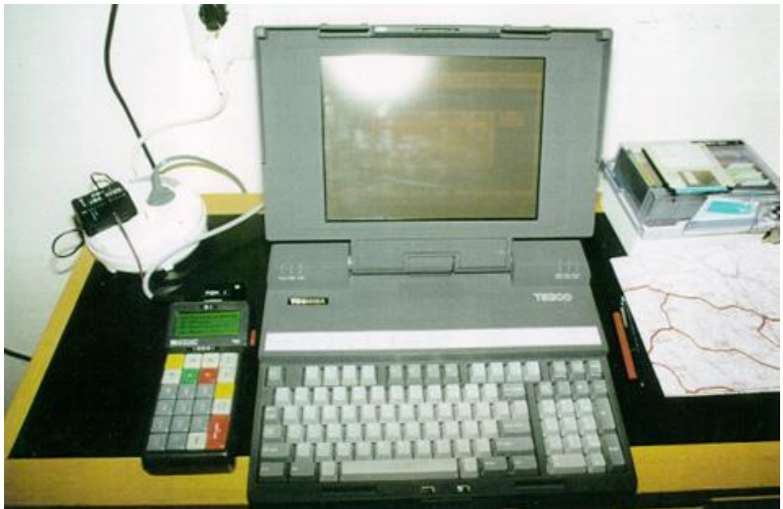
Figure 24: Dumping the daily Swedish levelling data from the field computer to a PC with a 35 Mb hard disc at the hotel in 1990.
