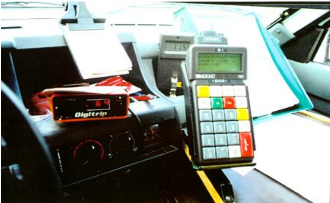
Figure 21: Interior from a Swedish ML instrument car 1995, with the data logger, Digitrip distance meter and air temperature display.
