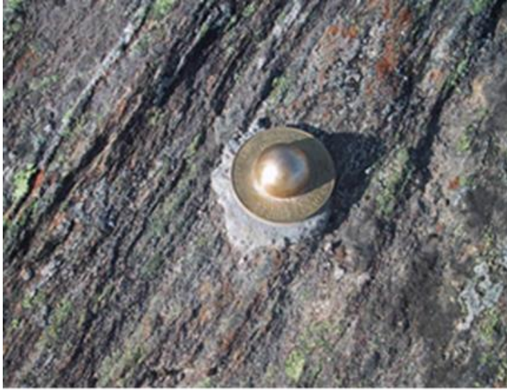
Figure 1: A Norwegian benchmark in bedrock.
