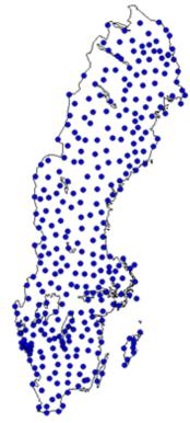
**Figure 1.7:** *The approximately* 300 *SWEREF points from the RIX 95 project, which totally included 9029 points.*
