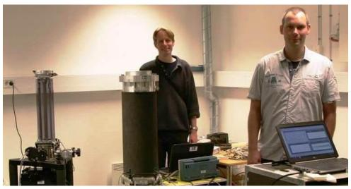
**Figure 2.2:** *Calibration of the super-conducting gravimeter with two absolute gravimeters (both Micro-g LaCoste FG5) in May 2014.*
