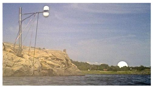
**Figure 2.3:** The GNSS tide gauge installation, with one zenith-looking and one nadir-looking antenna (covered by hemispherical radomes), at the Onsala Space Observatory. The radome of the 20 metre radio telescope in the background.
