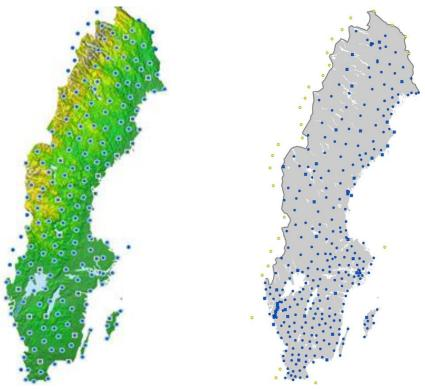
**Figure 1.5:** The SWEPOS network by the time for the previous NKG General Assembly in 2010 to the left and by the time for the 17th NKG General Assembly in September 2014 to the right. Squares indicate class A stations and dots indicate class B ones. Stations in neighbouring countries used in the SWEPOS Network RTK Service are also marked, but stations from other service providers are not marked.
